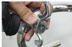
6. Put the plastic washer (9) and the stainless cover (10) on the shift lever.
