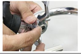
7.Set the fixing bolt ① to the pivot axis to fix the shift lever
